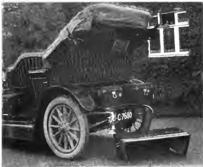
FIG. 4.—How space under rear seat is utilized to advantage.
